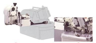
THIS PULLER IS UNABLE TO INSTALL ONTO OVERLOCK MACHINE WITH EITHER VERTICAL OR HORIZONTAL AUTOMATIC THREAD-CHAIN CUTTER.
